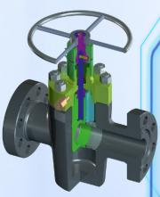
This type of valves is used in the oilfield industry for drilling and production operations for nominal pressures of 210, 350, 700 and 1050 bar (3000, 5000, 10000 and 15000 PSI) and nominal dimensions from 2 1/16 until 7 1/16.
