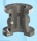
These are full-opening, straight-bore spools, flanges and the passing inside diameters are designed according to API spec.6A. The side outlets of casing spools are available on studded, LP or TBG threaded, or extended flange. Valve-removal threads standard in studded flanged outlets to provide ability to replace or add a full opening valve under pressure Valve removal plugs are available.
