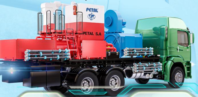
The cementing units are mobile units designed to perform cementing, fracturing, pressure balancing, extinguishing and acidizing operations at the wells.
