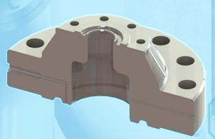
Single studded adapter flanges PET-THA-EN type are standard, used along with type PET-TH-EN extended-neck tubing hangers. They provide a secondary seal, and a test port that allows seal test of the connection.
