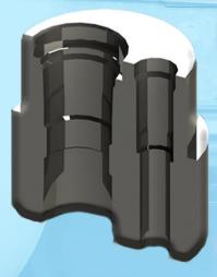
PET-TH-ESP tubing hanger is used in conjunction with electrically driven submersible pumps, (ESP's). The hanger is prepared with two ports: one port designed to accept a single production tubing string; the second port is designed to accommodate the electrical supply cable that powers the pump; designs have been completed that also allow down-hole control valves and/or fiber optic instrumentation lines.
